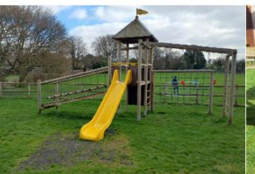
Finding: There are openings leading from platforms in excess of 1.0m in height to steep play elements and no hand supports complying with grip or grasp are provided, in contravention of BS EN 1176 Part 1: 4.2.9.4
