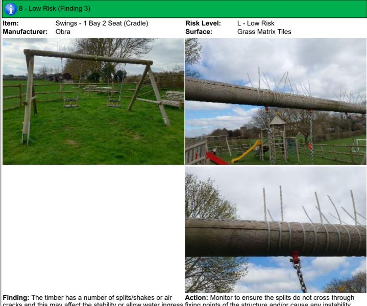
**Finding:** The timber has a number of splits/shakes or air **Action:** Monitor to ensure the splits do not cross through cracks and this may affect the stability or allow water ingress fixing points of the structure and/or cause any instability which will accelerate the rotting process
