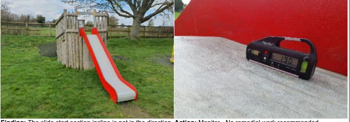
**Finding:** The slide start section incline is not in the direction **Action:** Monitor - No remedial work recommended of travel; it should slope towards the direction of the sliding surface to meet the requirements of BS EN 1176 Part 3
